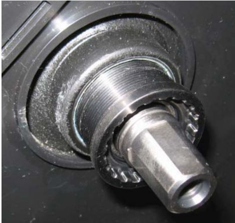
Install Right Side Cartridge 1-2 threads.
