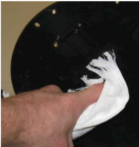
Wipe Shell threads with towel to remove any oil.
