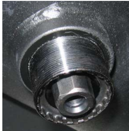
Install Left Side Cup 1-2 threads.
