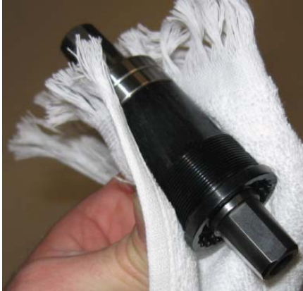
Wipe Bottom Bracket Cartridge with towel to remove any oil.
